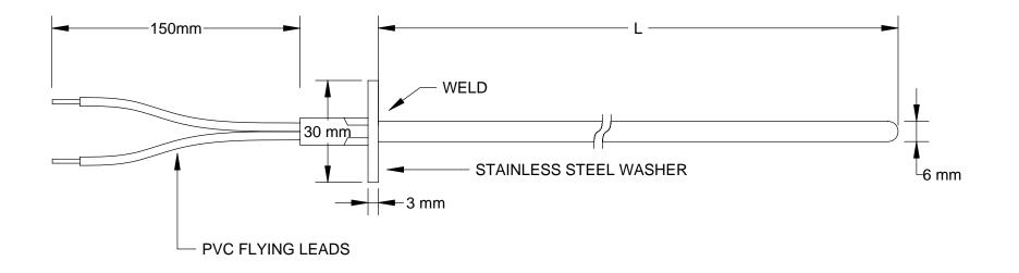
TYPE K THERMOCOUPLE FIXED WASHER ASSEMBLY
